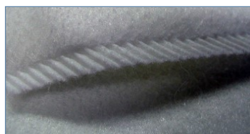
precision welding seam
